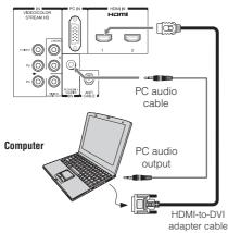
The HDMI input can accept and display VGA, SVGA, XGA, WXGA, SXGA, 480i (60Hz), 480p (60Hz), 720p
