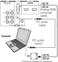
To use a PC, set the monitor output resolution on the PC before connecting it to the TV. The PC IN terminal can accept and display VGA, SVGA, XGA, WXGA and SXGA signal formats. For detailed signal specifications (rsp page 56).
