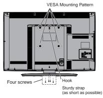
**CAUTION:** Always place the TV on the floor or a sturdy, level, stable surface that can support the weight of the unit. To secure the TV, use a sturdy strap from the hook(s) on the rear of the TV to a wall stud, pillar, or other immovable structure. Make sure the strap is tight, secure, and parallel to the floor.
