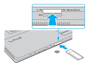
Be sure to hold the Memory Stick with the arrow pointing in the correct direction as you insert it into the slot. To avoid damaging your computer or the media, do not force the Memory Stick into the slot if you cannot insert it smoothly.
