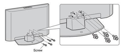
If an electric screwdriver is used, set the torque to tighten at approximately 1.5 N·m {15 kgf·cm}.
