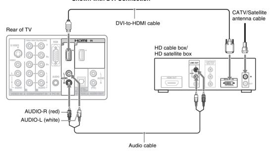
If the equipment has a DVI jack and not an HDMI jack, connect the DVI jack to the HDMI IN 1 (with DVI-to-HDMI cable or adapter) jack and connect the audio jack to the AUDIO IN (L/R) jacks of HDMI IN 1. For details, see page 17.
