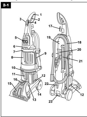
The assembled deep cleaner will look like the drawing. Model with SpinScrub™ hand tool is shown.
