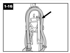
Insert top of bare floor tool (available at additional cost if not included with your cleaner) through "loop" on caddy. Slide tool down into place.
