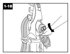
Pull tool down and outward. To reposition the tool, reverse this procedure.
