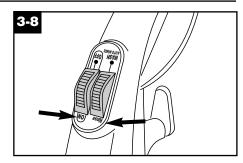
11. If you would like to rinse the carpet with water only, set Rinse Setting switch to **RINSE** (Fig. 3-8). Repeat steps 7-9. In this setting, rinsing will be done on both forward and reverse strokes.
