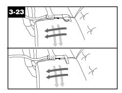
Make no more than 2 passes with the solution or rinse over any one area to prevent over-wetting and damage to fabric.
