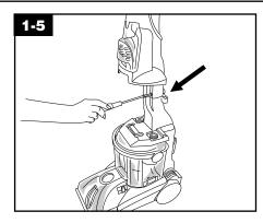
Push bolts into holes on front of handle. If bolts will not go through hole easily, handle is not pushed completely down.
