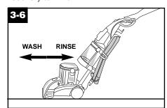
10. For best results, use straight, parallel strokes as shown in the diagram below. Overlap strokes by 1 inch to help prevent streaking.
