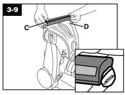
2. With foam strip (C) (located under the netting) in position as shown, place attachment on front of nozzle (D). Make sure arrow on end of attachment points in the direction as shown.
