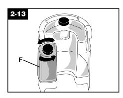
To fill detergent container (F), turn cap counterclockwise and remove cap.
