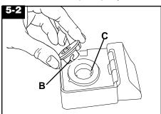
3. Align slots (B) on cap with tabs (C) in opening.
