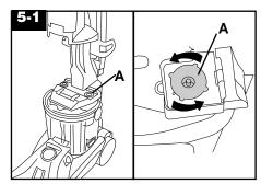
2. Turn valve cap (A) counterclockwise and remove.
