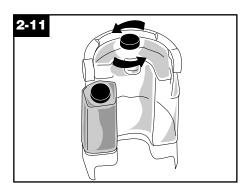
Carry tank to a sink. Turn tank cap counterclockwise and remove cap.
