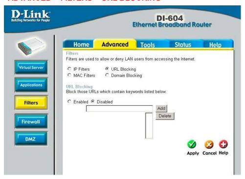
**URL Blocking** is used to deny LAN computers from accessing specific web sites by its URL. A URL is a specially formatted text string that defines a location on the Internet. If any part of the URL contains the blocked word, the site will not be accessible and the web page will not display.
