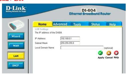
LAN is short for Local Area Network. This is considered your internal network. These are the IP settings of the LAN interface for the DI-604. These settings may be referred to as Private settings. You may change the LAN IP address if needed. The LAN IP address is private to your internal network and cannot be seen on the Internet.
