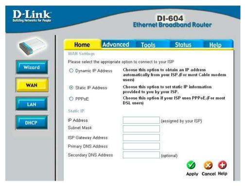
Choose Static IP Address if all WAN IP information is provided to you by your ISP. You will need to enter in the IP address, subnet mask, gateway address, and DNS address(es) provided to you by your ISP. Each IP address entered in the fields must be in the appropriate IP form, which are four IP octets separated by a dot (x.x.x.x.x). The Router will not accept the IP address if it is not in this format.
