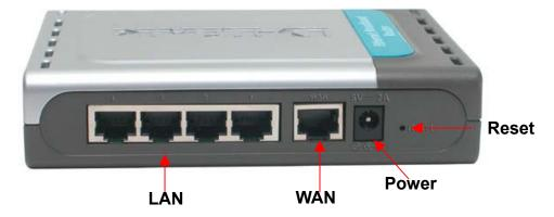
**Reset** Used to restore the DI-604 back to factory default settings.
