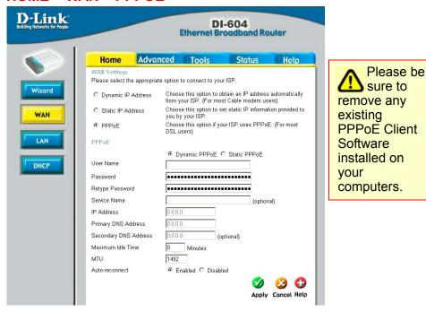
Choose PPPoE (Point to Point Protocol over Ethernet) if you're ISP uses PPPoE connection. Your ISP will provide you with a username and password. This option is typically used for DSL services. Select Dynamic PPPoE to obtain an IP address automatically for your PPPoE connection. Select Static PPPoE to use a static IP address for your PPPoE connection.
