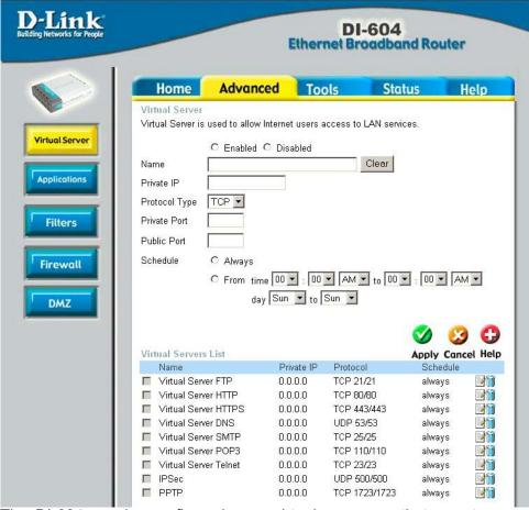
The DI-604 can be configured as a virtual server so that remote users accessing Web or FTP services via the public IP address can be automatically redirected to local servers in the LAN network.
