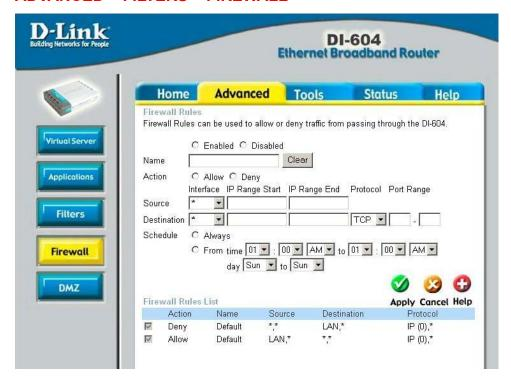
**Firewall Rules** is an advance feature used to deny or allow traffic from passing through the Broadband Router. It works in the same way as IP Filters with additional settings. You can create more detailed access rules for the DI-604. When virtual services are created and enabled, it will also display in Firewall Rules. Firewall Rules contains all network firewall rules pertaining to IP (Internet Protocol).
