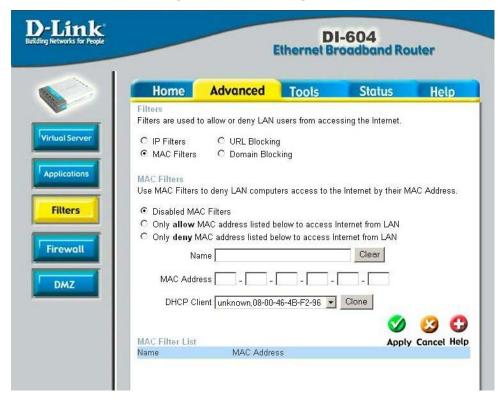
Use **MAC Filters** to allow or deny LAN computers by their MAC addresses from accessing the Internet. You can either manually add a MAC address or select the MAC address from the list of clients that are currently connected to the Broadband Router.
