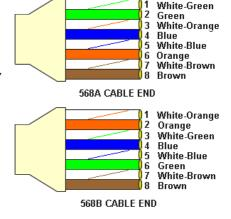
both sides, it is straight-through cable. If one side has opposite wiring, it is a crossover cable.
