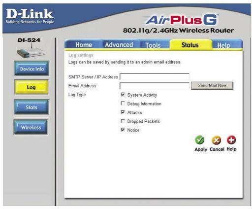
Not only does the Broadband Router display the logs of activities and events, it can setup to send these logs to another location.
