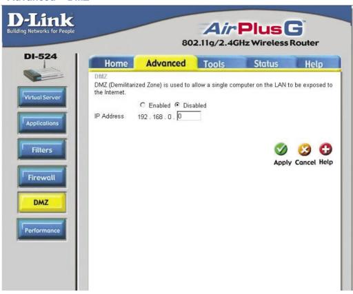
If you have a client PC that cannot run Internet applications properly from behind the DI-524, then you can set the client up for unrestricted Internet access. It allows a computer to be exposed to the Internet. This feature is useful for gaming purposes. Enter the IP address of the internal computer that will be the DMZ host. Adding a client to the DMZ (Demilitarized Zone) may expose your local network to a variety of security risks, so only use this option as a last resort.
