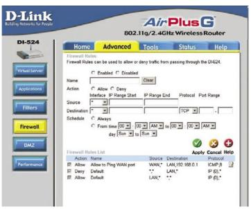
**Firewall Rules** is an advanced feature used to deny or allow traffic from passing through the DI-524. It works in the same way as IP Filters with additional settings. You can create more detailed access rules for the DI-524. When virtual services are created and enabled, it will also display in Firewall Rules. Firewall Rules contain all network firewall rules pertaining to IP (Internet Protocol).
