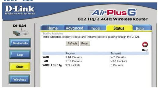
The screen above displays the Traffic Statistics. Here you can view the amount of packets that pass through the DI-524 on both the WAN and the LAN ports. The traffic counter will reset if the device is rebooted.
