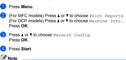
If the IP Address on the Network Configuration List shows 0.0.0.0, wait for one minute and try again.
